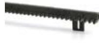
ROA6 (for RB400) M4 25x20x1000 mm slotted nylon rack with metal insert for gates weighing up to 500 kg. Pc/pack 10
